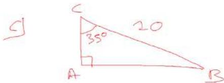
$$\begin{aligned}\cos 35^\circ &= \frac{AC}{BC} \text{ donc } AC = BC \times \cos 35^\circ \\ &= 10 \times \cos 35^\circ \text{ cm} \\ &\approx 8,2 \text{ cm \u00e0 1 mm pr\u00e8s}\end{aligned}$$
